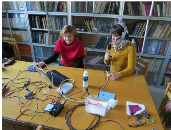
Figure 4.1. Example of ultrasound recording session using helmet to fix ultrasound transducer to the chin. Image provided by the MTA-ELTE Lendület Lingual Articulation Research Group
